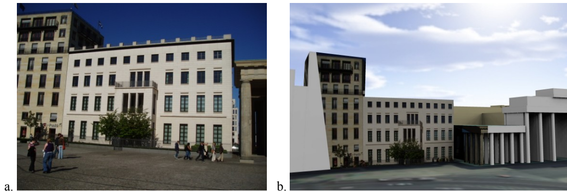
Fig. 17: Projecting a photograph (a) onto multiple facades (b) using the worldToTexture transformation. The photograph does not cover the left facade completely. Thus, the texture appears to be clipped. Texture wrapping is set to “none” (source: Senate of Berlin, Hasso-Plattner-Institute).
